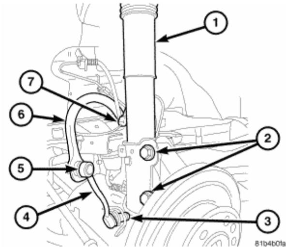
Camber angle adjustments involve changing the position of the knuckle at the strut base ([Refer to 2 - SUSPENSION/WHEEL ALIGNMENT - SPECIFICATIONS](#)).
