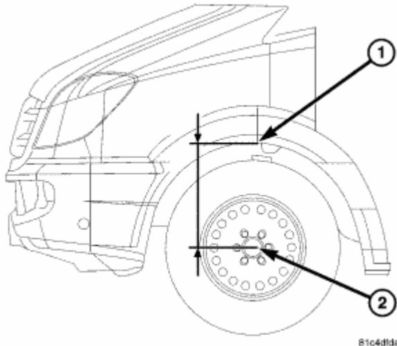
**NOTE:** Before each alignment check, measure the distance between the wheel center (2) and wheel well housing (1) on either side of the vehicle. Verify that it is between minimum and maximum values given. If so, the alignment check can be performed. If not, adjust the height of the front of the vehicle as necessary using the cradle until the distance is within specification. ([Refer to 2 - SUSPENSION/WHEEL ALIGNMENT - SPECIFICATIONS](#)) .
